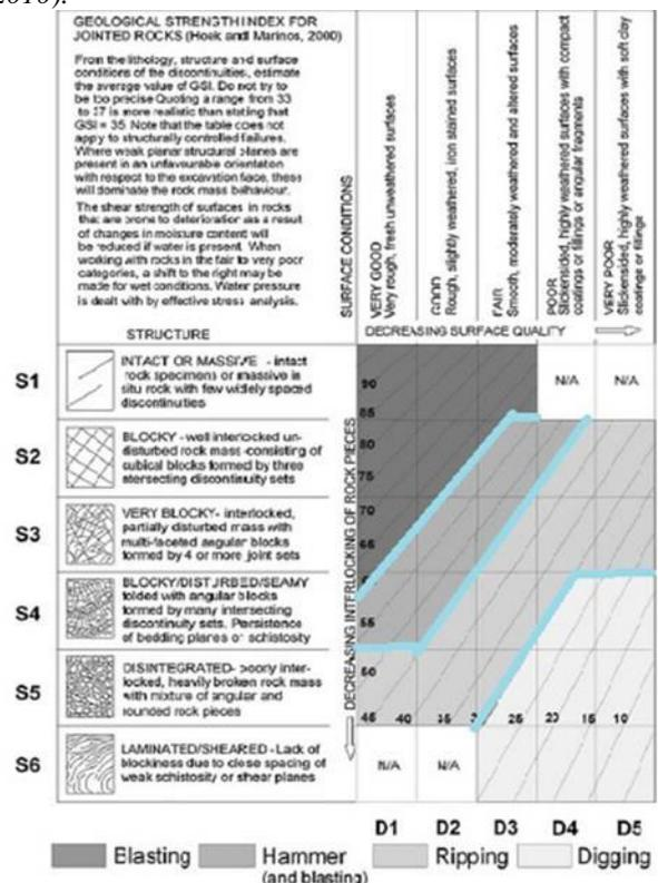
Fig 3: Rock Class and suitable rock breaking methods (insitu strength more than 70 MPa) (Tsiambaos G et al, 2010).
