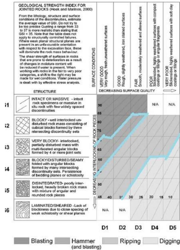
Fig 2: Rock Class and suitable rock breaking methods (insitu strength less than 70MPa) (Tsiambaos G et al, 2010).
